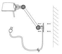
2. Installation on junction box in the wall; the lamp can be switched on with the light switch on the lamp socket.
